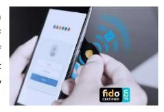
Feitian ePass FIDO<sup>®</sup>-NFC employs high-performance NXP secure elements. Besides generating strong keys pairs for FIDO<sup>®</sup> U2F application, the JAVA smart card platform in the secure element also provides room for other applications. An OATH one-time password application is also pre-installed in Feitian ePass FIDO<sup>®</sup>-NFC.
